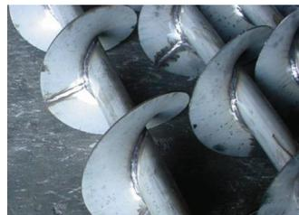
Standard Finish w/ Fully Welded Seams
